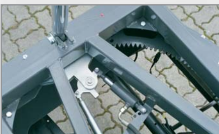
Infinitely variable, hydraulically releasable live ring lock
