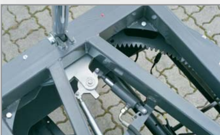
Infinitely variable, hydraulically releasable live ring lock
