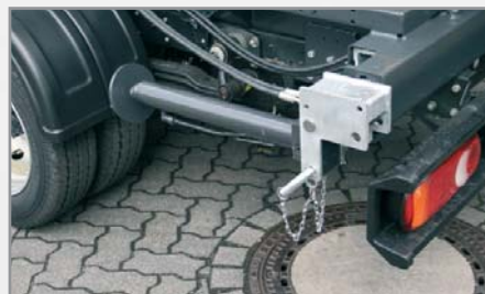
Hydraulic supports 90° foldable (transport position)
