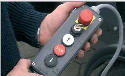
Electric control via cable operation
