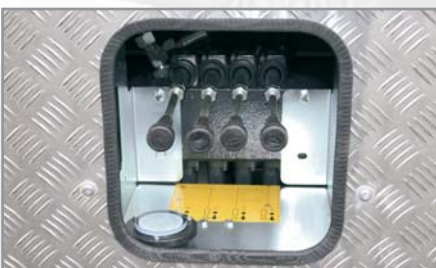
Control stand for hydraulic supports
